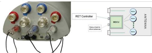
The MDCU is fully inserted inside the bottom of the antenna and leaves more room for spacing between co-axial connectors. For all Amphenol internal RET systems, when an MDCU module is installed in an antenna, all the tilt indicators remain visible and manual change of the tilt is still possible (manual override, the controller will read the new tilt setting).
